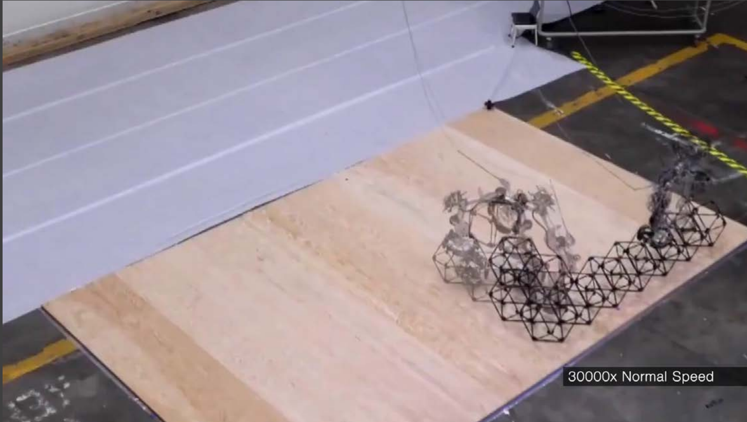
A structure is robotically built using the ARMADA voxel structural elements and assembly robots
