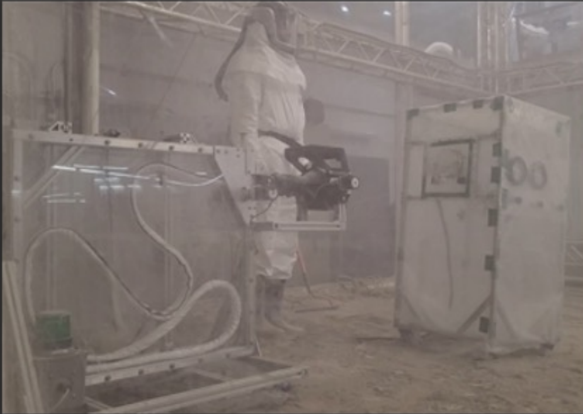
A dust tolerant umbilical is tested in extreme dusty conditions
